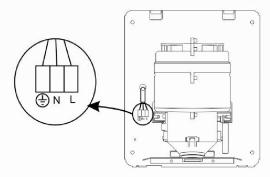
3. Drill four holes on the wall where the hand dryers will be installed, the diameter of the hole is 7mm and the deep is 40mm. Put in the expansion pipe into the hole. Then fix the machine on the wall with screws.
