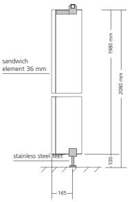
For a floating appearance, the connecting parts must be stably attached to the front. Please note our special technical information.
