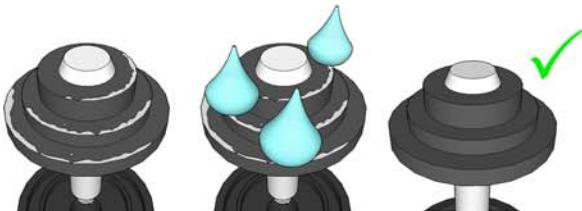
6) Place the parts in the correct position, put everything together and open the water supply
