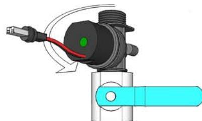
3) Remove the solenoid valve from the housing
